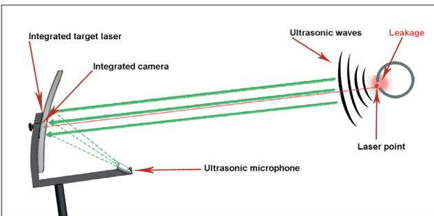
By focusing the ultrasonic waves in the parabolic mirror, even the smallest leaks of 0.8 l/min (approx. € 8 p.a.) can be located with pinpoint precision ( $\pm 15$  cm) at a distance of up to 10 to 15 m.
